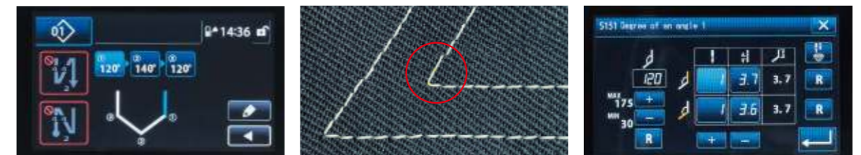
*1 Seams where the inside of the corner stitching has floated *2 Active tension setting screen
