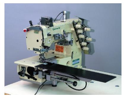
High performance & de-skillizing sleeve hemming workstation, which had given breakthrough in world's T-shirt manufacturing, is now upgraded with additional features.
