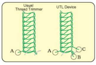
UTL device cuts the under thread at two points of "A" and "B" as the above picture. As "C" becomes the thread end, it prevents the seam from unraveling, unlike the case only "A" is cut at the end of the
