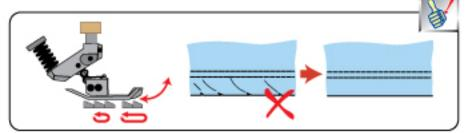
Walking Presserfoot releases unnecessary pressure on the fabric sewn and helps your work finished without waves and twists. Also, it is effective in lightening tracks of presser foot on dark-colored fabric.
