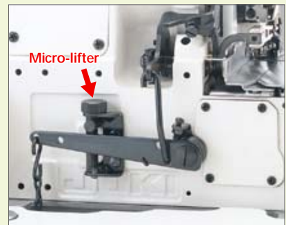
Bottom and top differential-feed micro adjustment mechanism
