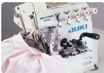
● Gathering MO-6714D-BE6-327/S162 (S162: Swing-type gathering device, manual-lever operated)
