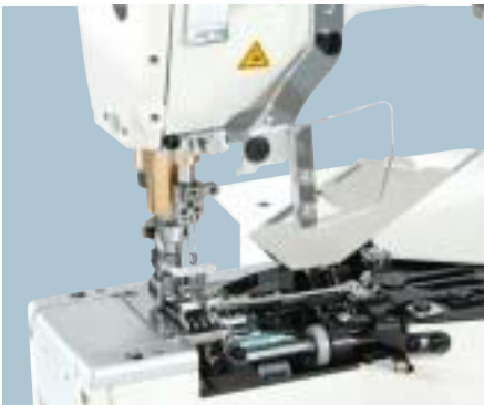
Pneumatic type bottom thread trimming device
